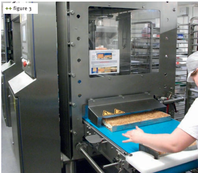
++ figure 3 Feeding the machine manually at Geiping (visible on the left: the Rittal HD housing with pitched roof etc. & control panel)
