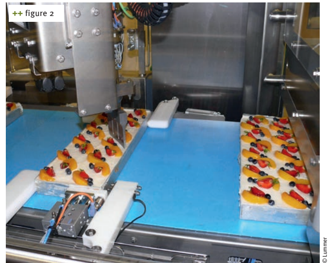
++ figure 2 Ultrasonically assisted cutting for a perfect cut – lengthwise or crosswise
